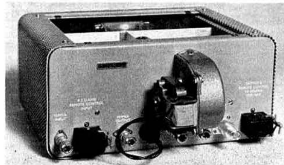
The rear view of the new Green and Davis Ltd. 70CM1000 40-90 watt 432 Mc/s tripler-amplifier. The blower provides forced air cooling for the QAV03-20A tripler and the QAV03-20A or QAV06-40A p.a. The 70CM1000 can be driven by a 2m transmitter, the Green and Davis 2M15-20A Falcon, which is built in a matching cabinet, or the 2M1000 being suitable. A heavy-duty aerial change-over relay is incorporated, but this can be bypassed for duplexing systems.
